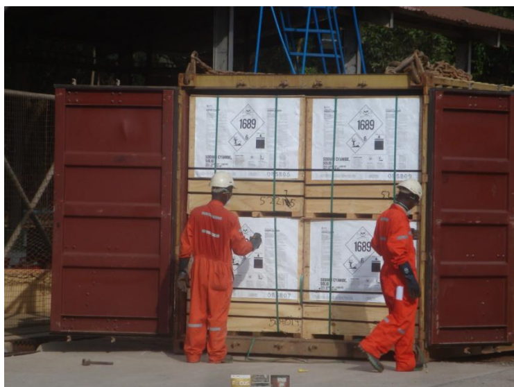
Workers should take protective measures when opening containers carrying cyanide.
