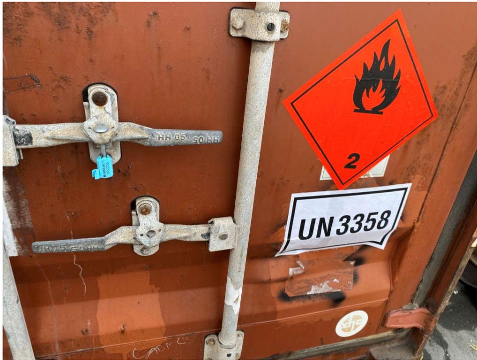
**Photo 9:** View of container with UN number and hazard category references as well as seal.
