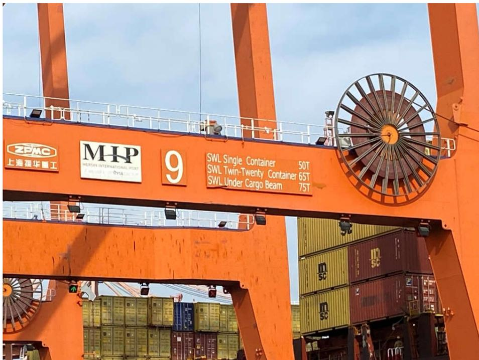
**Photo 20:** View of MIP # 9 SSG crane nominal lifting capacity information.
