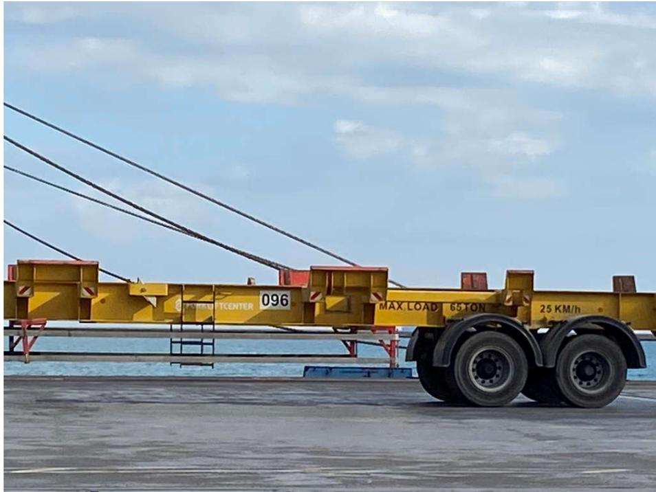
**Photo 19:** View of MIP #96 truck-trailer maximum load capacity rating information.
