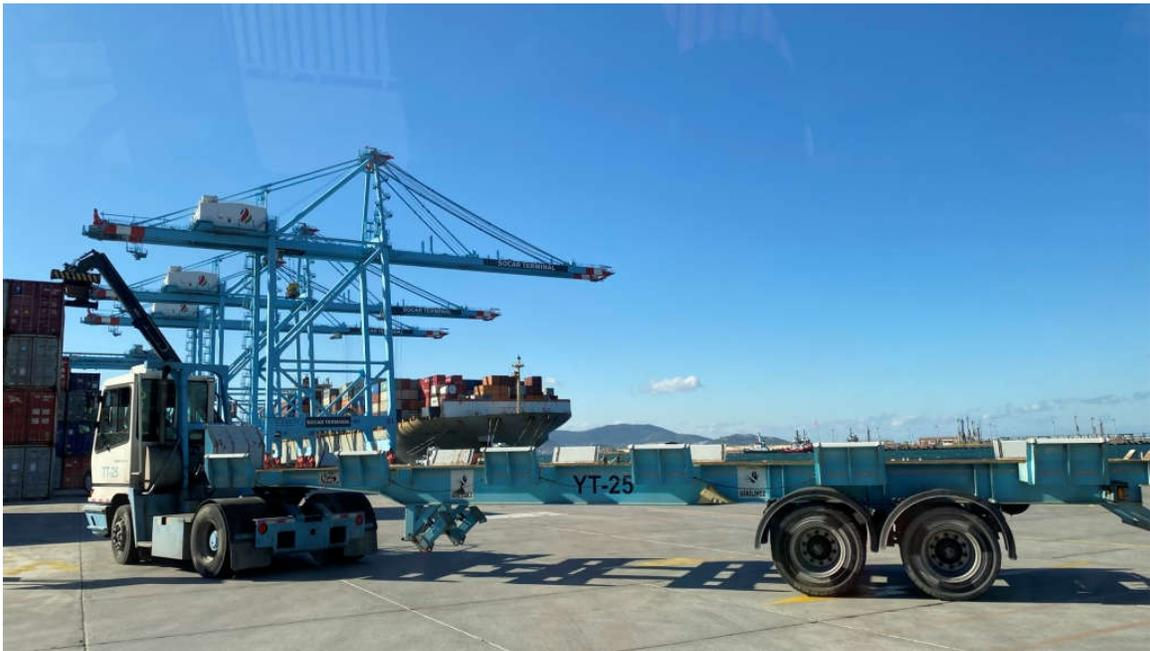
**Photo 8:** View of SOCAR Terminal tractor trailer used for container handling between wharf and interim storage area.
