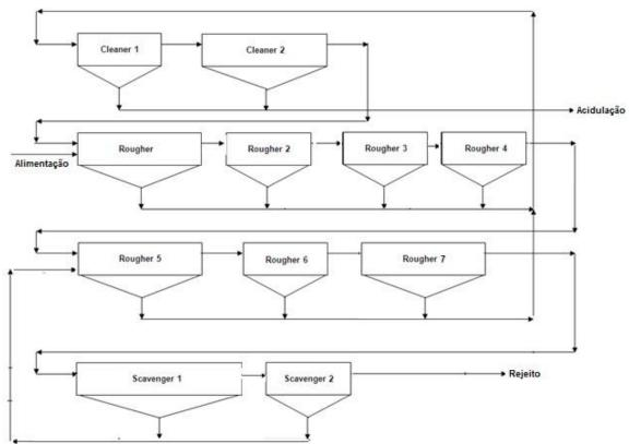
The rougher flotation concentrate is removed and will feed the cleaner flotation circuit that consists in 3 smart cells and 2 conventional cells.
