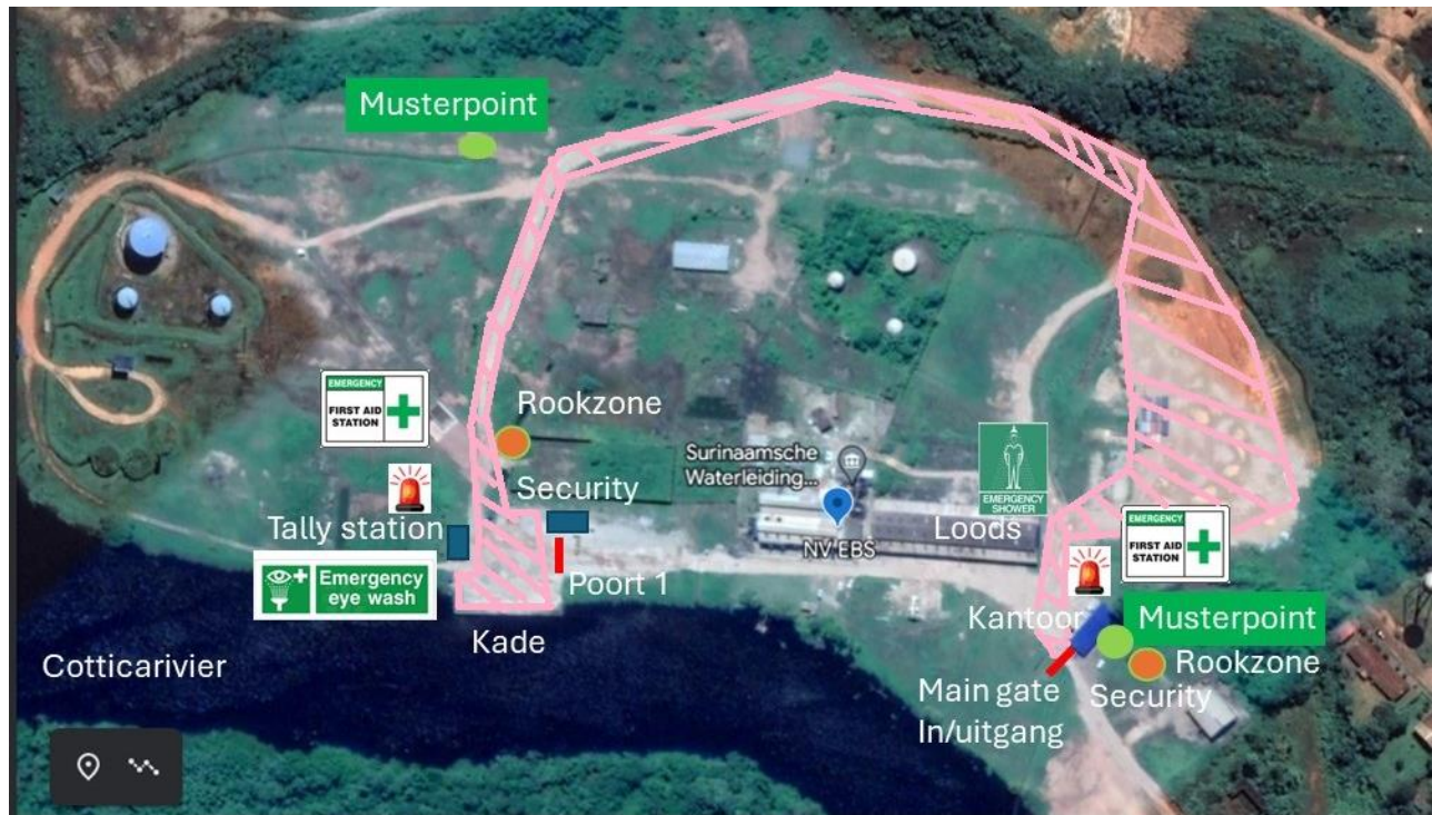
Figure E: Moengo Port Safety Facilities and Areas for Sodium Cyanide Transportation and Handling (Pink)
