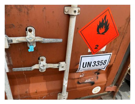
Photo 9: View of container with UN number and hazard category references as well as seal.
