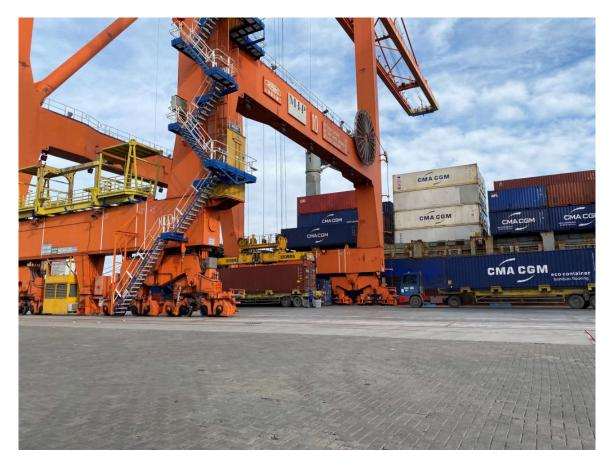
Photo 4: View of SSG (Ship-Shore Gantry) crane and MIP truck-trailer container loading.
