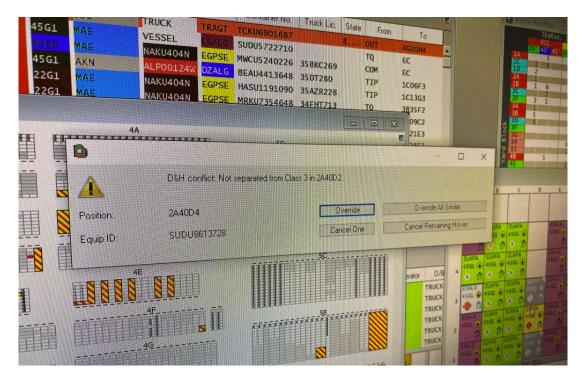
Photo 19: View of NAVIS N4 software and operator storage request denial functionality.
